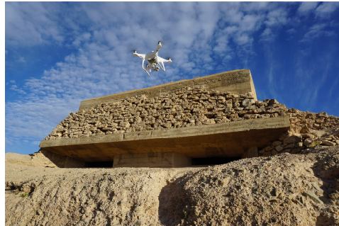
Fig. 5. DJI Phantom 4 Pro drone taking photographs of the machine gun bunker of Alhama de Murcia.
