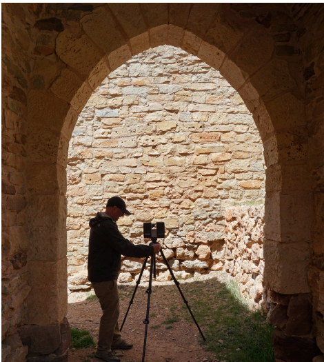
Fig. 4. FARO Focus3D S70 laser scanner working in Molina de Aragón castle.
