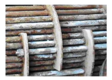
Figure 5. Image of scaling in a shell and tube heat exchanger [19].
