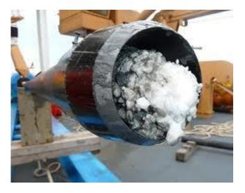
Figure 6. Gas hydrate formation in a pipe [23].
