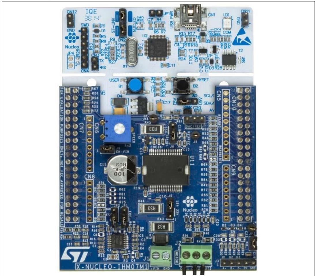
1. The interconnection between the X-NUCLEO-IHM07M1 and the STM32 NUCLEO boards has been designed for a full-compatibility with a lot of control board and no modification of solder bridges is required.
