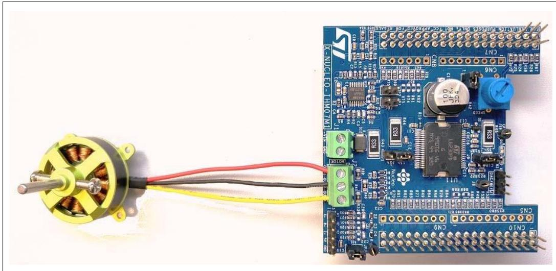
3. Select the jumper configuration on the power board to choose the desired control algorithm (6-step or FOC) as described below:
