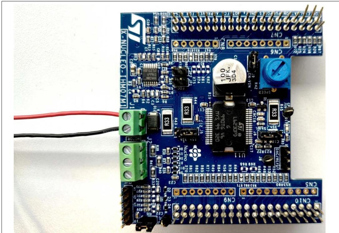
1. The red cable is VCC, the black one is GND.
