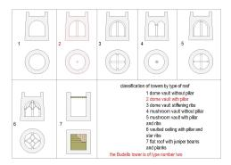
Fig. 2. Tower construction models; the Budello tower model is two type.
