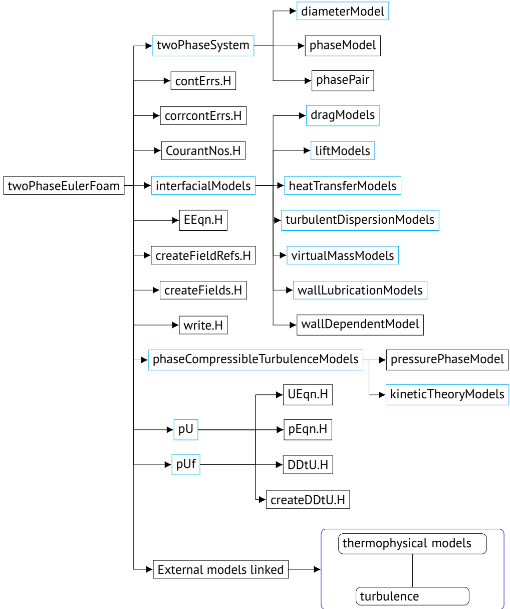
Figure 5.15: Built-in solver twoPhaseEulerFoam structure.
