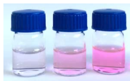
Figure 3. Visual changes observed for S2 suspensions in acetonitrile before and after exposure to 0.25 and 0.5 ppm of \text{NO}_2 gas (from left to right). The picture shows the color of the corresponding acetonitrile solutions after elimination of the nanoparticles by centrifugation.
