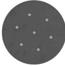
Fig. 5.1. Seven- core MCF cross section [94]
