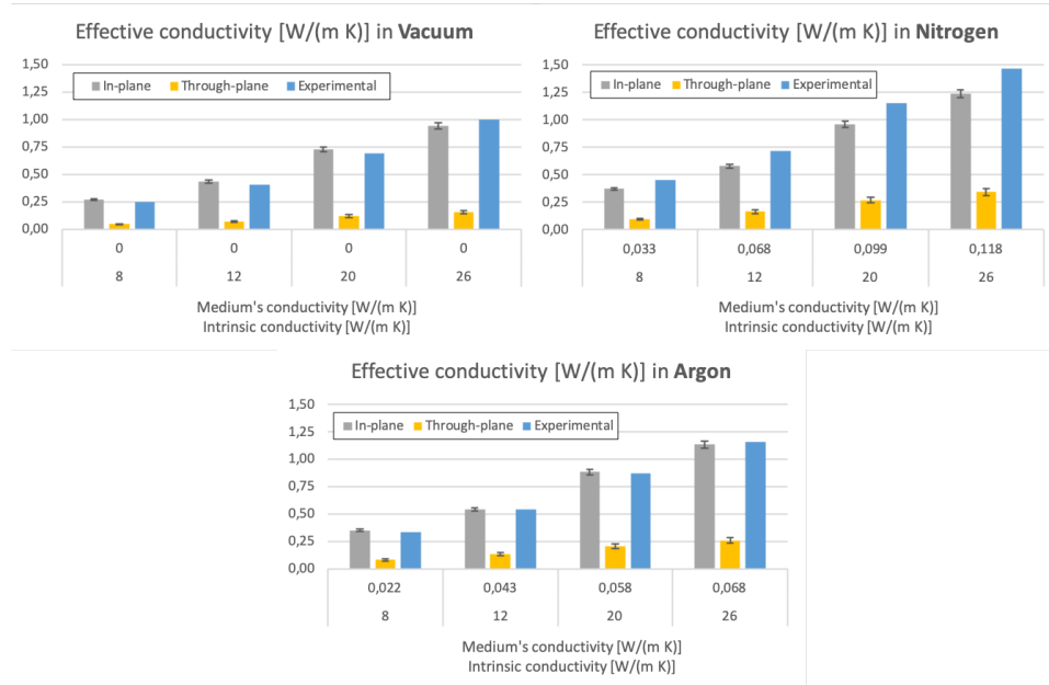
Figure 5.2: Comparison of experimental vs. computationally-obtained values for the effective thermal conductivity of CALCARB® CBCF 18–2000 as a function of the conductivity of the medium and the fibers. Error bars displayed from the results of Section 4.2.3.
