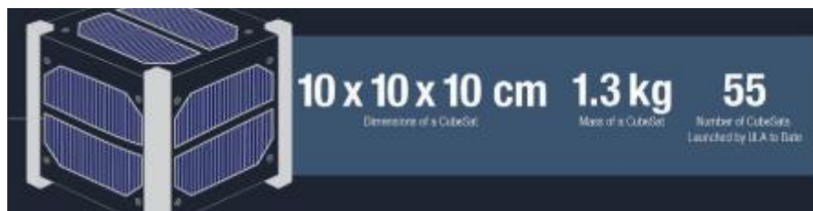
Figure 1 Main specifications of the CubeSat
