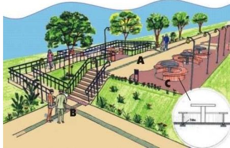
Figure 3: Open space with two alternatives to access different heights: ramp and stairs (Bins Ely, Souza, Domeles, Wan Dall Junior, & Koelzer, 2006).
