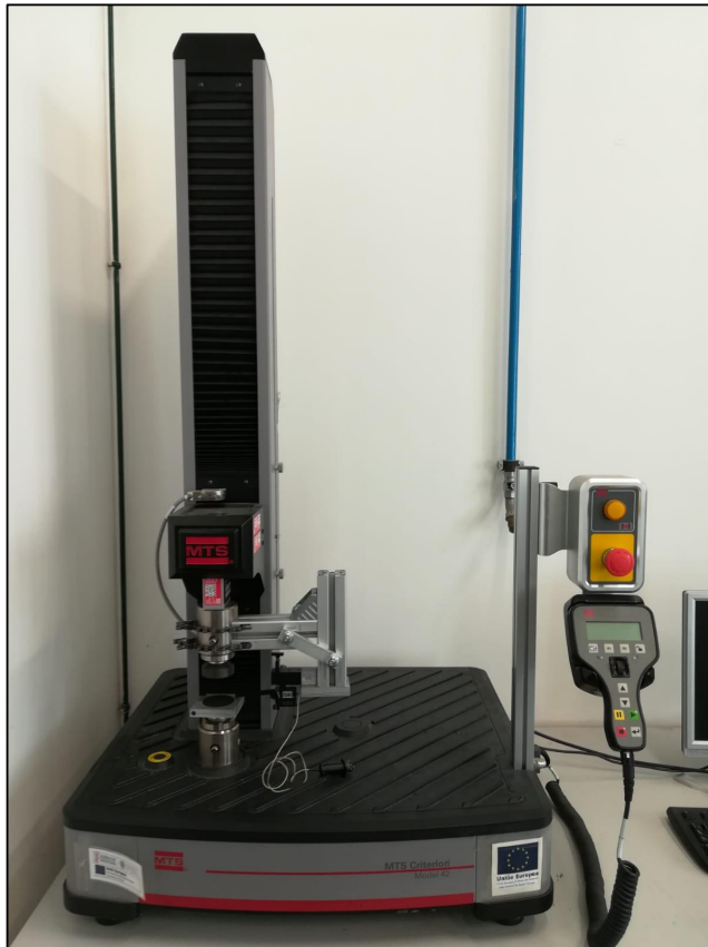
Figure 3.1: Electromechanical testing machine used for experimental testing: MTS Criterion c42.
