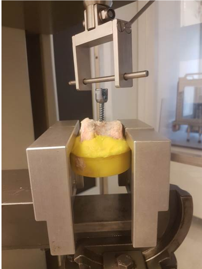
Figure 5.15: Pull-out test montage. It can be distinguished the rotative device to ensure uniaxial test conditions.
