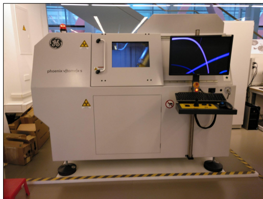
Figure 2.4: V|Tome|X s 240 \mu CT scanner used for high resolution images acquisition for sets A and B (CENIEH, Burgos, Spain).
