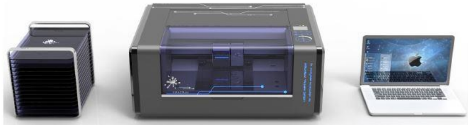
Fig. 20: Photo of the liquid metal printer based on the tapping-mode technique at room temperature.
