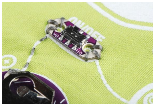
Image 1 – Conventional conductive yarn sewing. [12]
