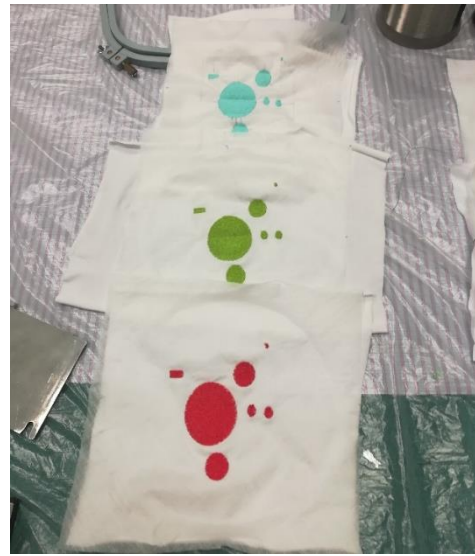
Image 25 – Prototypes with embroidered sensor simulation
