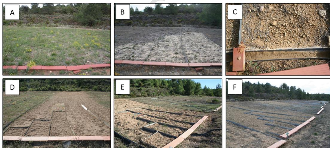
**Fig. 2.** View of the plots. A: Straw covered plot in spring; B: Straw covered plots in winter; C: view of the runoff collector; D: Control plot in summer after the ploughing; E: Control plot at the end of summer; F: View of the Control plot in winter.
