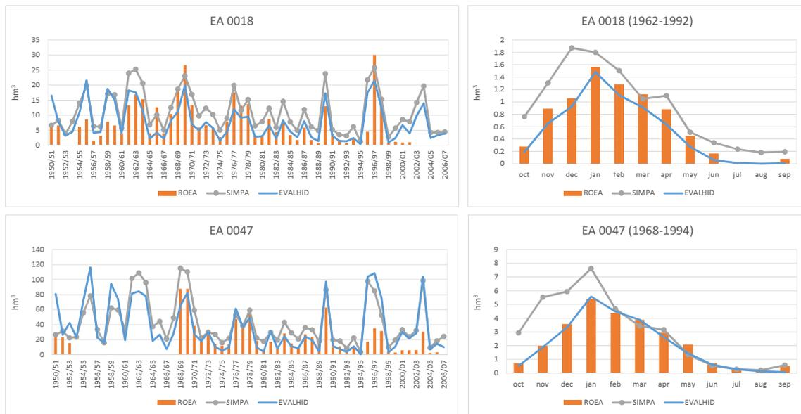
Figure 6. Comparison between EVALHID and SIMPA results with the flows registered in the gauging stations EA 0018 and EA 0047 ( $\text{hm}^3$ ) (ROEA means gauging stations official network)
