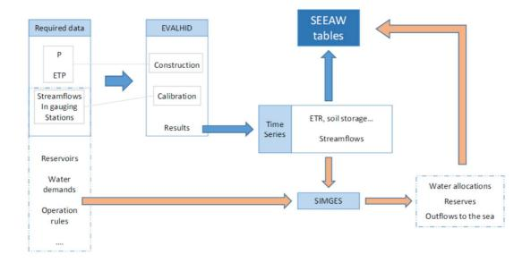
Figure 2. Process to obtain SEEAW tables by using EVALHID and SIMGES tools (Source: EC (2015))
