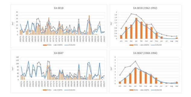
Figure 6. Comparison between EVALHID and SIMPA results with the flows registered in the gauging stations EA 0018 and EA 0047 (hm<sup>3</sup>) (ROEA means gauging stations official network)
