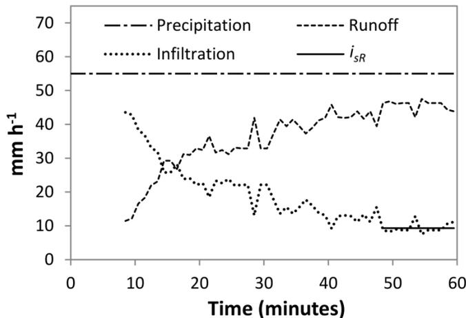
**Figure 2.** Illustrative example of a 1-hour simulated rainfall on a 0.56 m diameter plot at 55 mm h<sup>-1</sup> rainfall intensity. The infiltration curve was drawn by subtracting the runoff rate from the intensity. The experimental steady-state infiltration rate,  $i_{sR}$  (9.3 mm h<sup>-1</sup>), was estimated considering the last thirteen data points
