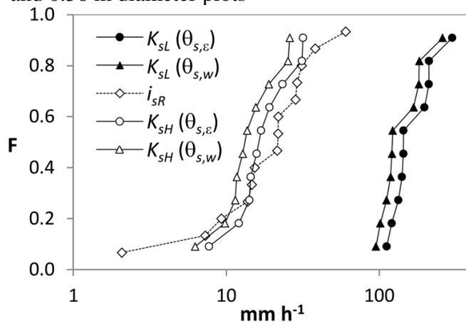
**Figure 5.** Cumulative empirical frequency distribution of the steady-state infiltration rates of the rainfall simulation experiments,  $i_{sR}$  (for both the 0.09 and 0.56 m diameter plots), and the saturated soil hydraulic conductivity,  $K_s$  (for both  $\theta_s$  values), obtained by pouring water into the cylinder from two different heights (L and H runs).
