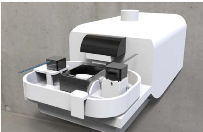
Figure 2. Automatic positioning device for cutting three-dimensional tissue in a sample of living or fixed tissue. The figure shows the three-dimensional model assembled and joined to a vibratome.
