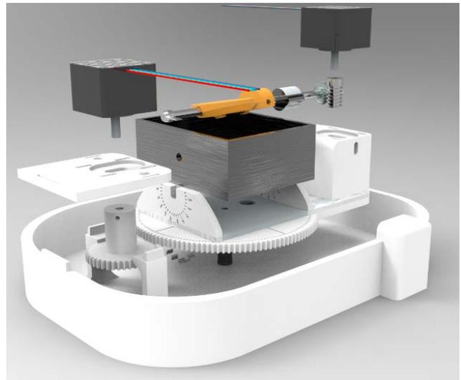
Figure 3. Automatic positioning device for cutting three-dimensional tissue in a sample of living or fixed tissue. The figure shows the three-dimensional model disassembled.
