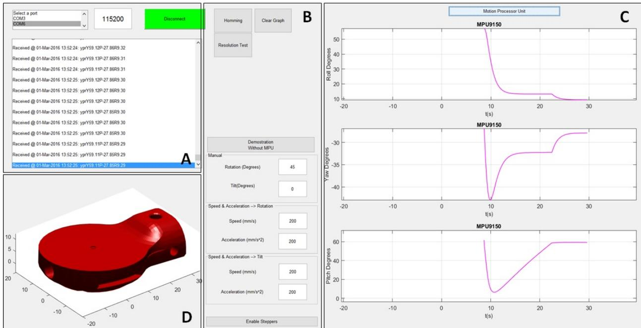
Figure 6. Graphical user interface. This Graphical User Interface (GUI) was made to control each movement of the system and to visualize all of orientation data. At zone A communications settings can be changed to communicate with the system properly. The device setting is provided in zone B. The sensor measurements can be shown in the C zone. Inside of D zone, a real time representation of the Sample's platform is shown while the system is working.
