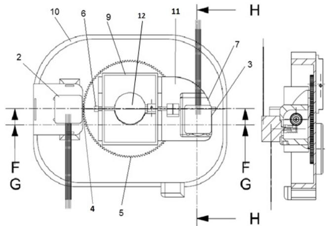
Figure 4. Schematic illustration of the 3D positioning system. The figure on the left shows the top view of the plant and on the right a side view showing the cutting G is depicted. 1-Sample platform, 2-Rotation engine, 3-Angular engine, 4-Rotation power gear, 5-Rotation gear, 6-Shaft, 7-Gearbox, 9-Inner container, 10-Ice container, 11-Structural support, 12-Samples platform.[16]
