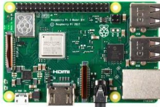
Figura 2.2 Placa Raspberri Pi 3B+
