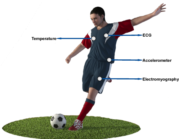
Figure 1 Illustration of sensors placed on a football player, considering accelerometer, electrocardiogram (ECG), electromyography (EMG), and temperature sensors (see online version for colours)
