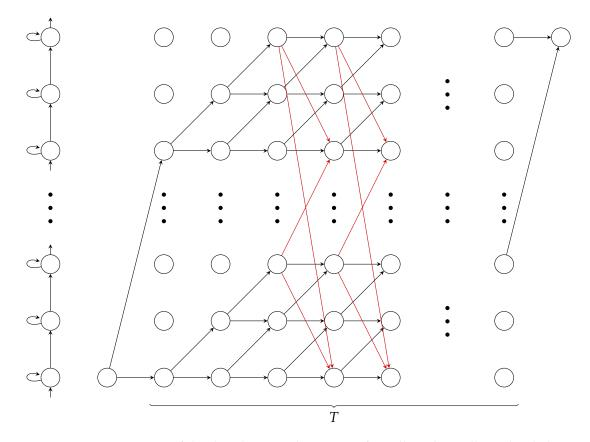
**Figure 2.8:** Representation of the decoding step by means of a trellis. This trellis is divided into *T* sections, being *T* the number of frames or acoustic features from the sample. Black arrows indicate the usual HMM transitions, whereas red arrows indicate transitions which may appear, depending on both the dictionary of words and whether cross-word acoustic units are considered or not.
