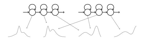
**Figure 4.3:** Graphical representation of senone sharing by the HMM states. The emission probabilities of each HMM state are modeled by the senones, and each senone may model one or more HMM states' emission probabilities.
