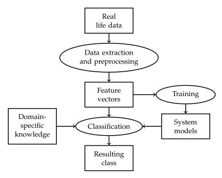
**Figure 2.1:** Design of the basic structure of a pattern recognition system. Circles design actions, while squares reference available data or information at each step.
