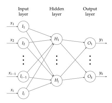
**Figure 2.2:** General structure of a neural network. In this neural network,  $M_0 = i$ ,  $M_1 = j$  and  $M_2 = k$ . Each neuron *m* is connected with every neuron *n* of the following layer *n* by a weight, which is usually represented as  $\theta_{nm}$ .
