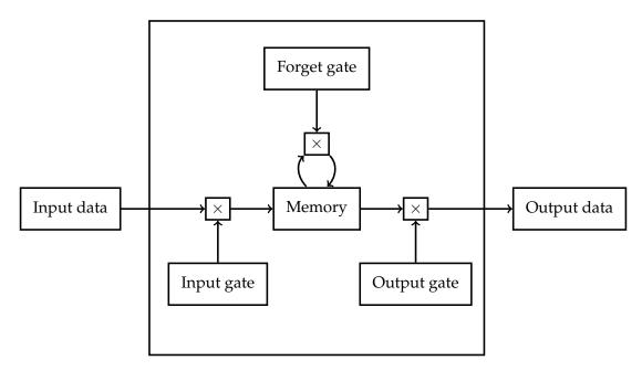
**Figure 2.3:** Basic schema of an LSTM memory cell. Nodes labeled with  $\times$  denote the multiplication operation performed on the inputs that arrive to such node.
