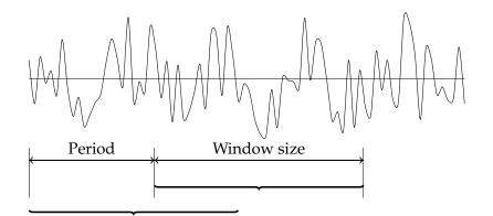
**Figure 2.5:** Graphical representation of the window size and period parameters when extracting windows from an audio signal. The values that TLK uses are 25 ms for the window size and 10 ms for the period, yielding a total of approximately 100 windows per second.
