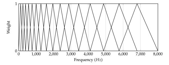
**Figure 2.6:** Mel filter bank consisting of 16 different filters. Each of the different filters corresponds to a triangle.
