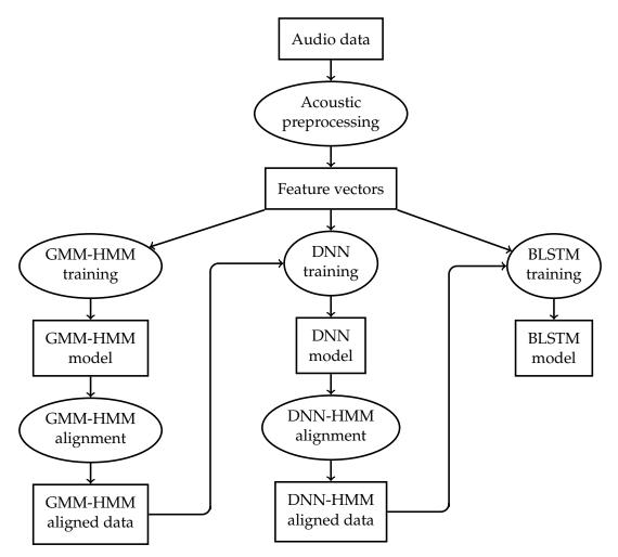
**Figure 4.1:** Basic sequence of actions performed in order to train the final acoustic models. Circles design actions, while squares reference available data or information at each step. This figure is best followed from left to right, and from top to bottom.
