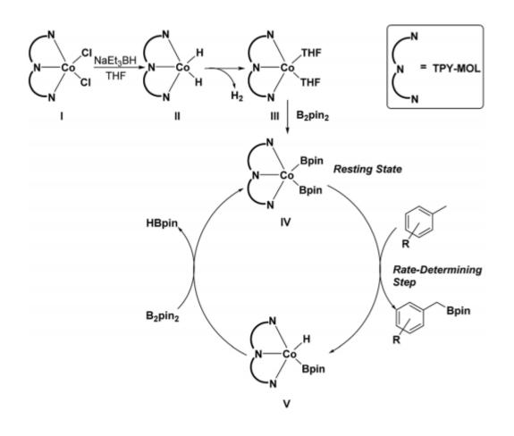
Figure 19. Proposed mechanism for the CoCl<sub>2</sub>.TPY-MOL catalyzed C-H borylation of arenes with B<sub>2</sub>pin<sub>2</sub>. Reprinted with permission from ref.50 Copyright 2018 Royal Society of Chemistry.
