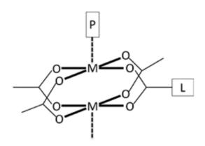
Figure 1. Illustration of the coordination geometry of paddle wheel building units in Ni<sub>2</sub>(BDC)<sub>2</sub>(DABCO). M stands for metal ion, L stands for bicarboxylate linker (BDC) and P is N-containing bidentate pillar linker (DABCO). Reprinted with permission from ref. 56. Copyright 2012, American Chemical Society.
