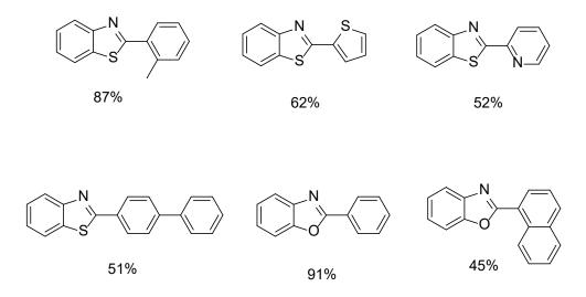
Scheme 6. Structure of heterocyclic compounds that can be obtained by C-H activation using  ${(H_3O)[Cu^I_2(CN)(TTB)_{0.5}]1.5H_2O}_n$  catalyst.
