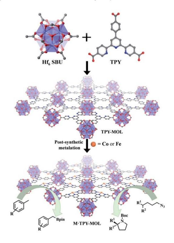
Figure 18. Structure of  $Hf_6$  secondary building units and TPY forming TPY-MOL followed by metalation to obtain M.TPY-MOLs (M=Co<sup>2+</sup> or Fe<sup>2+</sup>). Reprinted with permission from ref.50 Copyright 2018 Royal Society of Chemistry.
