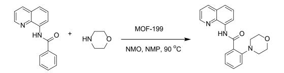
Scheme 17. C-N coupling between N-benzoyl-8-amino-quinoline and morpholine using MOF-199 as catalyst through oxidative C-H activation in NMP as solvent.
