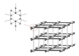
Figure 2. Pictorial representation of pillared-grid MOFs. Circles indicate bimetal paddlewheels, dark lines indicate grid-forming ligands (dicarboxylates) and lighter lines represent pillar ligands (diamines or diimines). Reprinted with permission from ref.57. Copyright 2007 Royal Society of Chemistry.
