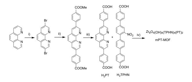
Scheme 28. Synthesis of mPT-MOF. Reaction conditions: (i) Br<sub>2</sub>, S<sub>2</sub>Cl<sub>2</sub>, pyridine, n-BuCl, reflux, 12 h; (ii) 4-methyl carboxyphenylboronic acid, Pd(PPh<sub>3</sub>)<sub>4</sub>, CsF, DME, 100 °C, 3 d; (iii) aq. NaOH, EtOH; (iv) ZrCl<sub>4</sub>, DMF, TFA, 100 °C, 5 d.
