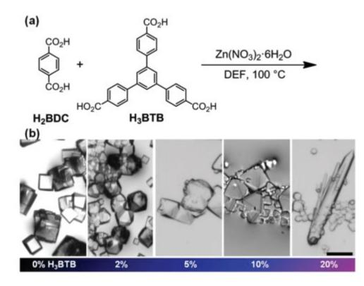
Figure 4. (a) Synthesis of BTB-incorporated MOF-5 crystals by addition of BTB to the reaction mixture of BDC and  $Zn(NO_3)_2.6H_2O$  (b) Photographs of crystals showing the dependence of the morphology upon the percentage of BTB in the feed (scale bar is 100 µm). Reprinted with permission from ref.35 Copyright 2011 American Chemical Society.
