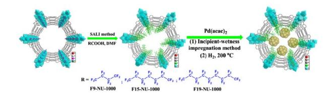
Figure 3. Schematic representation of introduction of perfluoroalkyl chains into the pores of NU-1000 by solvent-assisted ligand incorporation method followed by immobilization of the Pd NPs into the pores of perfluoroalkyl functionalized NU-1000 using incipient-wetness impregnation method. Reprinted with permission from ref.33 Copyright 2016 Elsevier.
