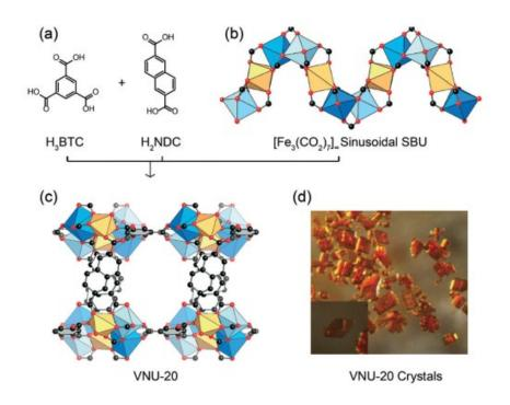
Figure 5. (a) Linker structures and (b) secondary building unit of VNU-20, (c) crystal structure of VNU-20 and (d) SEM image of VNU-20 crystals. Reprinted with permission from ref.36 Copyright 2018 Royal Society of Chemistry.
