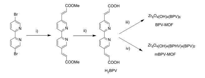
Scheme 27. Synthesis of BPV-MOF and mBPV-MOF. Reaction conditions: (i) methyl acrylate, Pd(OAc)<sub>2</sub>, P(o-tol)<sub>3</sub>, NEt<sub>3</sub>, DMF, 120 °C, 2 d; (ii) NaOH, EtOH, H<sub>2</sub>O, reflux; (iii) ZrCl<sub>4</sub>, DMF, TFA, 100 °C, 5 d; (iv) H<sub>2</sub>BPHV, ZrCl<sub>4</sub>, DMF, TFA, 100 °C, 5 d.
