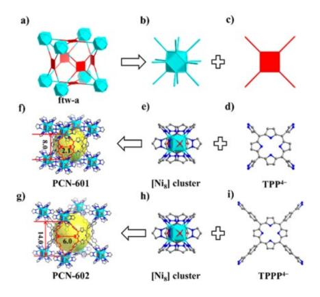
Figure 22. Reticular design and structure of PCN-602: (a) ftw-a topological net; (b) 12connected node with  $O_h$  symmetry; (c) 4-connected node with  $D_{4h}$  symmetry; (d) TPP<sup>4-</sup> ligand; (e and h) [Ni<sub>8</sub>] cluster; (f) structure of PCN-601 (Ni atoms in the porphyrin center are omitted for clarity); (g) proposed structure of PCN-602; and (i) TPPP<sup>4-</sup> ligand. Reprinted with permission from ref.53 Copyright 2017 American Chemical Society.
