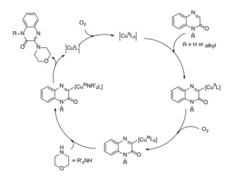
Figure 12. A possible mechanism for the C-N bond formation by Cu-CPO-27. Reprinted with permission from ref.42 Copyright 2017 Elsevier.
