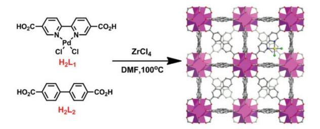
Figure 9. Synthesis of Pd(II)-doped UiO-67. The structure model (right) of Pd(II)-doped UiO-67 shows the incorporation of the L1 ligand into the framework. Reprinted with permission from ref. 39 Copyright 2014 Royal Society of Chemistry.
