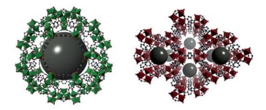
Figure 20. Pd NPs supported in MIL-101-NH<sub>2</sub>(Cr) cages (left, green) and MIL-88B-NH<sub>2</sub>(Fe) channels (right, red). Reprinted with permission from ref.51 Copyright 2016 Wiley.
