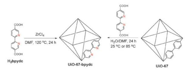
Figure 8. Preparation of UiO-67-bpydc either by direct synthesis or postsynthetic exchange method. Reprinted with permission from ref.38 Copyright 2014 Royal Society of Chemistry.
