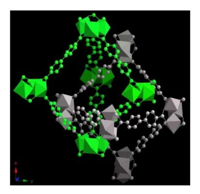
Figure 7. Organization of the two orthogonally interpenetrated trigonal bipyramidal building units in the crystal structure of Fe<sub>3</sub>O(BPDC)<sub>3</sub>. Reprinted with permission from ref. 60 Copyright 2012 American Chemical Society.
