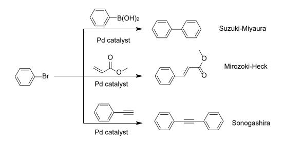
Scheme 1. Some conventional cross-coupling reactions catalyzed by Pd catalysts.
