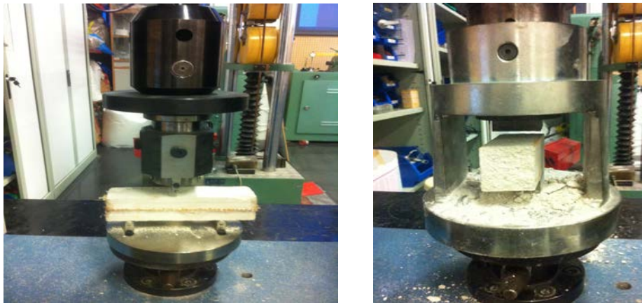
Fig. 2. Flexural and compression test
