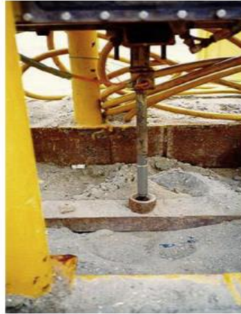
Figure 13. Cone penetration test. Source: Onshore structural design calculations
