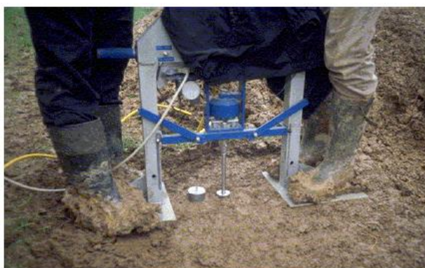
Figure 12. In-situ plate sinkage test. Source: Keller, 2004
