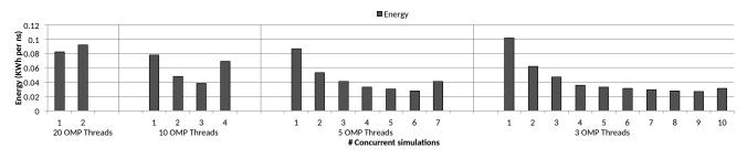
Figure 11. Energy per simulated ns required by GROMACS when several simulator instances share the GPU in the rCUDA server by leveraging the rCUDA middleware. Simulator configurations using either 20, 10, 5 or 3 threads are considered.
