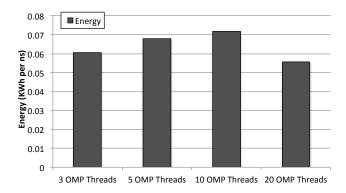
**Figure 7.** Energy per simulated ns required by GROMACS when several CPU-only instances are concurrently executed in the same node. Simulator configurations using either 3, 5, 10 or 20 threads are considered.
