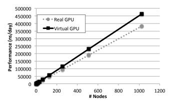
Figure 13. Aggregated throughput projection for a homogeneous cluster composed of n nodes where all the nodes own one GPU.
