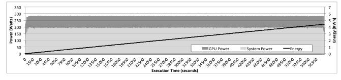
**Figure 9.** Instant power and accumulated energy along the execution time of the GROMACS simulator configured to use 10 threads with the molecules under study. Simulation was configured to last 200 ns of simulated time. Instant power is split into GPU power and system power.
