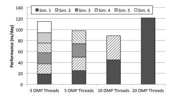
**Figure 6.** Throughput of the CPU-only MD simulations when several instances are concurrently executed in the same node. Simulator configurations using either 3, 5, 10 or 20 threads are considered.
