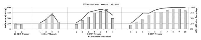
Figure 10. Throughput and GPU utilization when several instance of GROMACS share the GPU in the rCUDA server by leveraging the rCUDA middleware. Simulator configurations using either 20, 10, 5 or 3 threads are considered.
