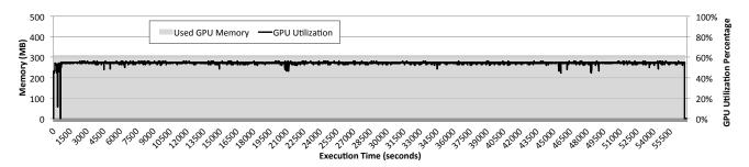
Figure 8. GPU memory and GPU utilization along the execution time of the GROMACS simulator configured to use 10 threads with the molecules under study. Simulation was configured to last 200 ns of simulated time.
