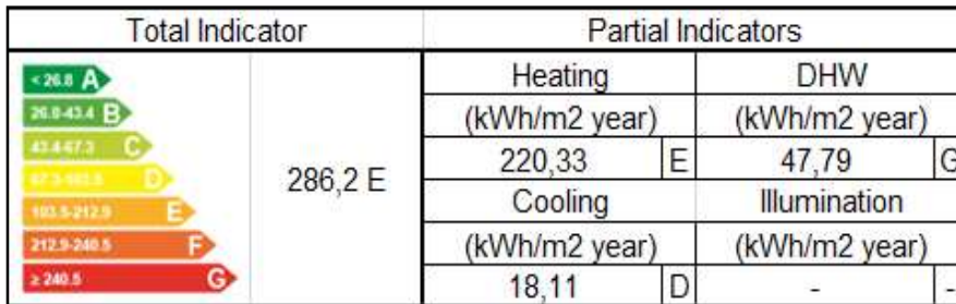
Figure 15: Energy rating of the building in non-renewable primary energy consumption. Source: CE3X
