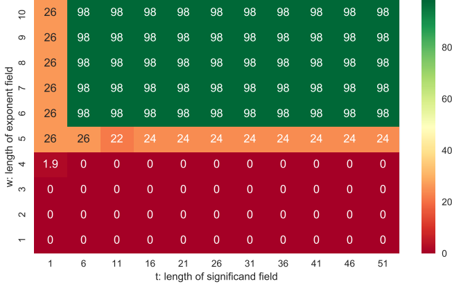
Fig. 4. Recognition accuracy of BLSTM when operating with type T_{w,t} . The baseline runs with T_{8,23} , which explains part of the plateau at around 98% accuracy. BLSTM operates close-to-perfect with further reduced formats.
