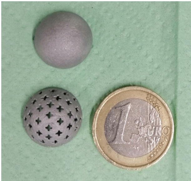
(a) Structures printed using aluminium as material.
