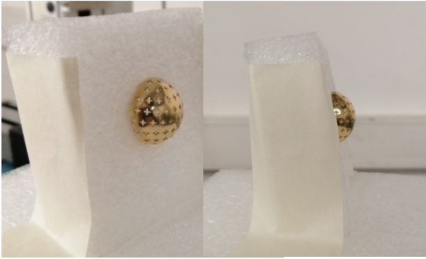
(a) FSS inserted in dielectric slab. The slab influence is eliminated from results by including it in reference measurement that is then subtracted.
