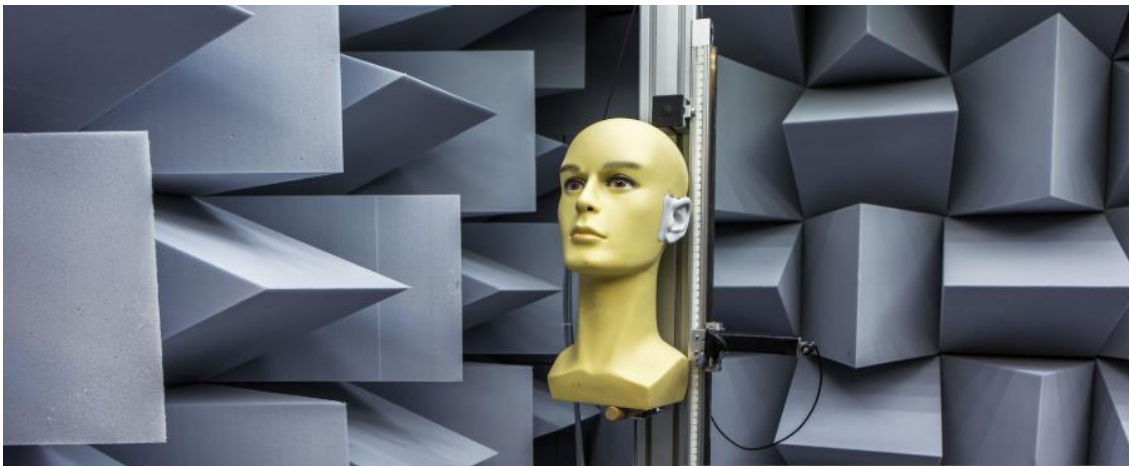
Figure 7 -Solid-dry Phantom in an anechoic chamber (Source: Bloomberg)
