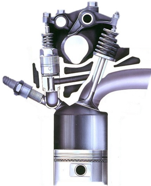
Figure 2.15: Combustion chamber layout of Honda CVCC engine [54]
