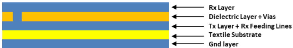
Figure 49. Cross-section of the 3DS-1 sensor. In addition to the 4 layers shown in Figure 48 the textile substrate between the ground plane layer and the Tx electrode layer can be observed.
