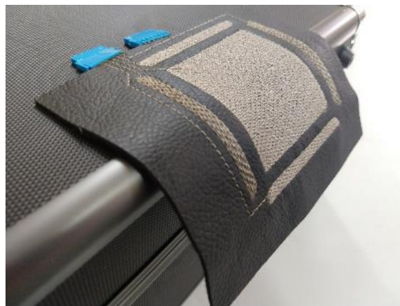
Figure 76. Flexible 3D Boosted sensor manufactured.
