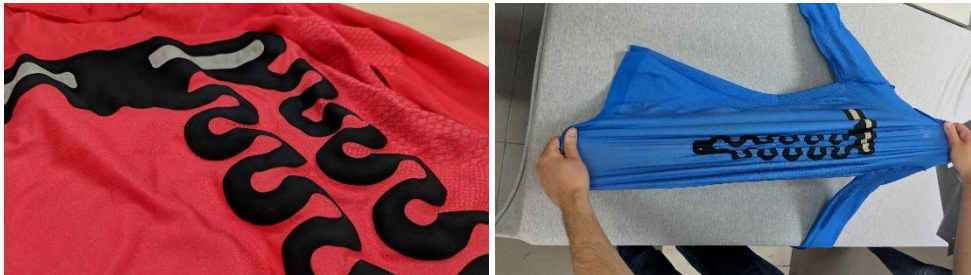
Figure 1. Textile electrodes to be used as ECG and EMG sensors. Source: AITEX.
