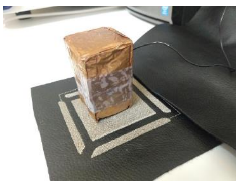
Figure 74. “Artificial hand” provided by Microchip made of styrofoam covered by copper and connected to ground.
