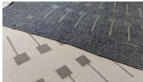
Figure 3. Conductive plates printed on fabric working as electrodes. Source: Screentex Project from AITEX.
