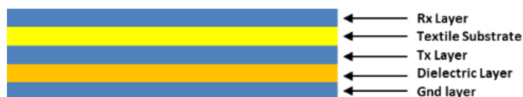
Figure 51. Cross-section of the 3DS-2 sensor. In addition to the 4 layers shown in Figure 50, the textile substrate between the Rx layer and the Tx electrode layer can be observed.
