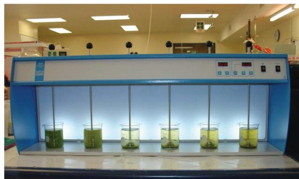
Illustration 11. A jar test unit for flocculation experiments
