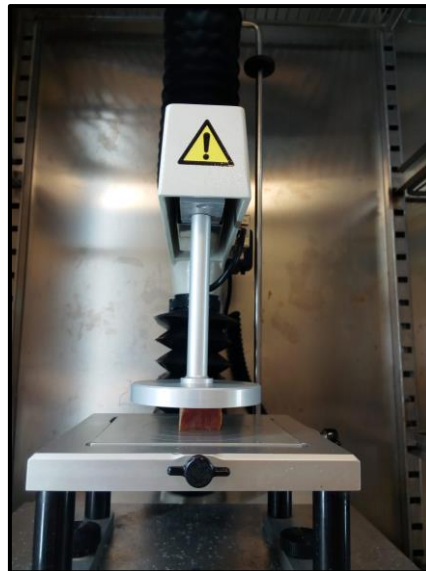
Figure 8. Stress-relaxation test carried out on dry-cured ham parallelepipeds with a cylindrical probe (75 mm of diameter).
