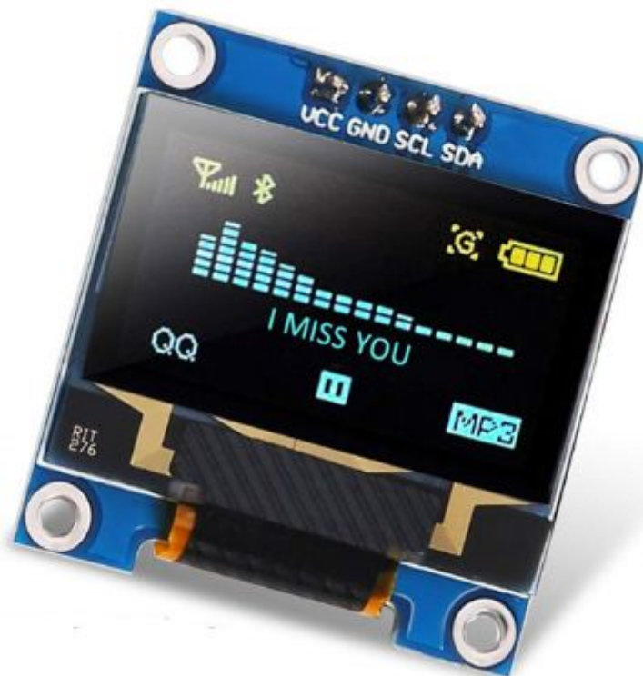
Figura 43. Panel OLED SSD1306
