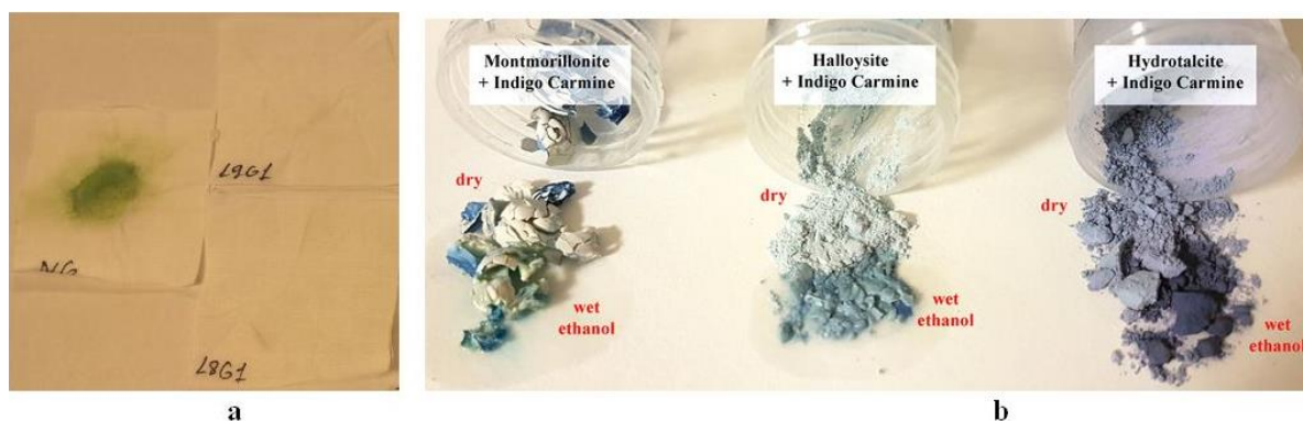
Figure 4. a) Cotton standard fabrics after wet rub test, with composite materials using epoxy bioresin and natural chlorophyll extract (NG), and hybrid pigments with laminar nanoclays under different synthesis conditions. b) Hybrid pigments samples with indigo carmine and montmorillonite, or halloysite, or hydrotalcite nanoclay.
