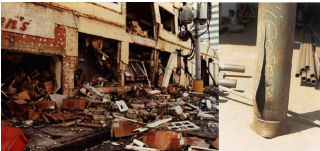
Figure 3.9: Explosions and cracks in cylinder by build-up pressure, respectively [19]
