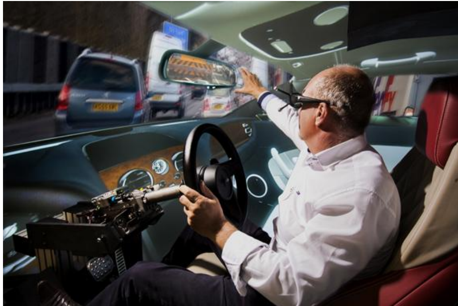
Figure 2.2 OPTIS VR lets Bentley Motors conduct ergonomic tests on virtual vehicle models
