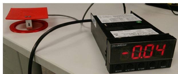
Fig. 4. Single point load cell (left) connected to the strain meter (right), which shows the strength applied to the red surface in newton.
