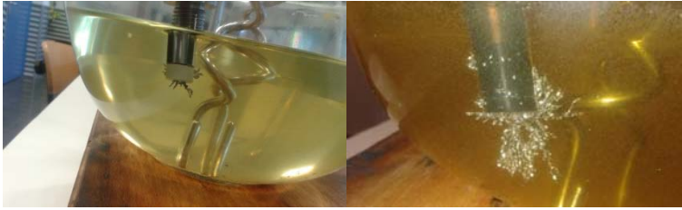
Figure 10. Image of mass trapped in the 1-2mm particles test for sensor A (left) and sensor B (right).
