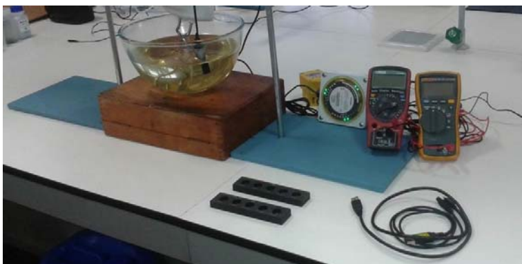
Figure 3. Experiment test rig, with the sensor installed and voltage meters to continuously control the results of the experiment.
