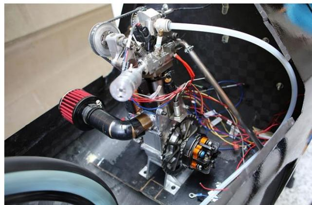
Figura 1.2: Sistemas de admisión de dos prototipos de la competencia Shell Eco-Marathon (Fuentes: <https://www.utoronto.ca/news/racers-start-your-fuel-efficient-engines> & <https://s.aolcdn.com/dims-shared/dims3/GLOB/crop/1030x692+150+148/resize/305x203!/format/jpg/quality/85/http://o.aolcdn.com/hss/storage/midas/6a7a42661aba493e6e11e0afb9bba441/200079664/shell-eco-marathon-2014-22.JPG>)
