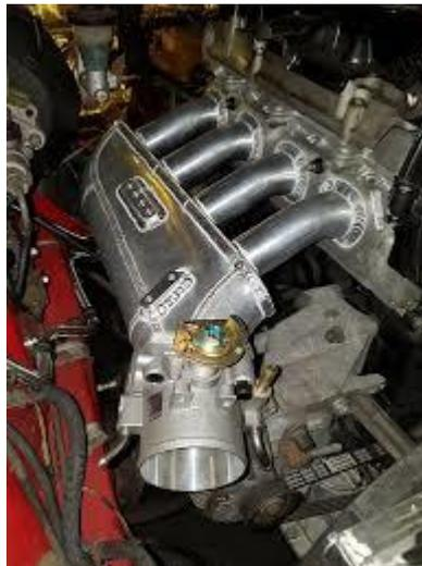
Figura 2.4.3: Plenum de admisión motor 3SGE Beams. (Fuente: <https://www.facebook.com/JustEngineManagement/posts/custom-made-plenum-to-suit-3sge-beams/996142047196237/>)
