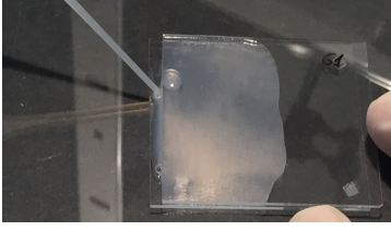
Fig. 6. Filling process of an LC cell by capillarity.
