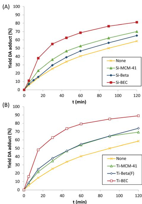
**Fig. 3** Catalytic activity for the Diels–Alder reaction using different silicate (A) and titanosilicate materials (B). Reaction conditions: 0.26 mmol 1,3-cyclohexadiene, 0.20 mmol *N*-methylmaleimide, 2 ml  $\text{CDCl}_3$ , 30 mg of catalyst, and  $T = 60$  °C.
