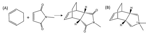
Fig. 1 DA reaction between 1,3-cyclohexadiene and *N*-methylmaleimide (A) and (3a*R*,4*S*,7*R*,7a*S*)-2,2-dimethyl-2,3,3a,4,7,7a-hexahydro-1*H*-4,7-ethanoindol-2-ium molecule as OSDA mimic of the DA adduct (B).
