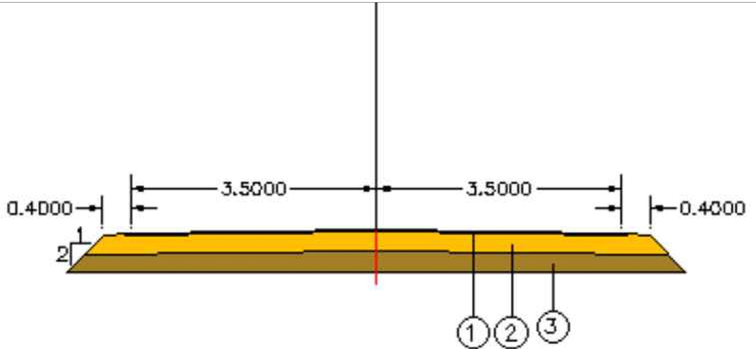
1. Capa de rodadura-5cm- AC22 surf S BC<sup>38</sup>
