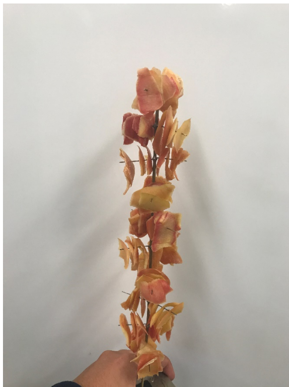
Figure 1. Apple peel distribution in the sample holder before being placed in the dryer
