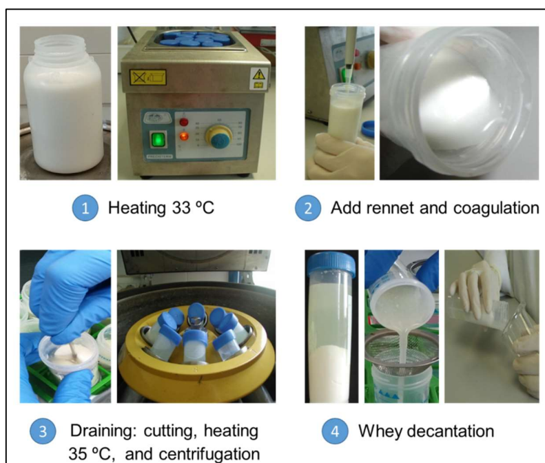
Figure 23. Cheese-making procedure at lab scale
