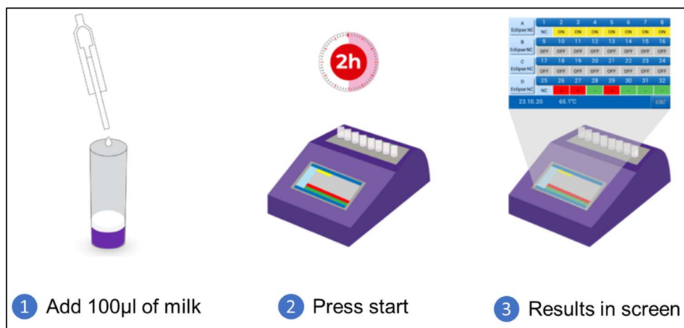
Figure 26. Analytical procedure of Eclipse Farm-eReader test
