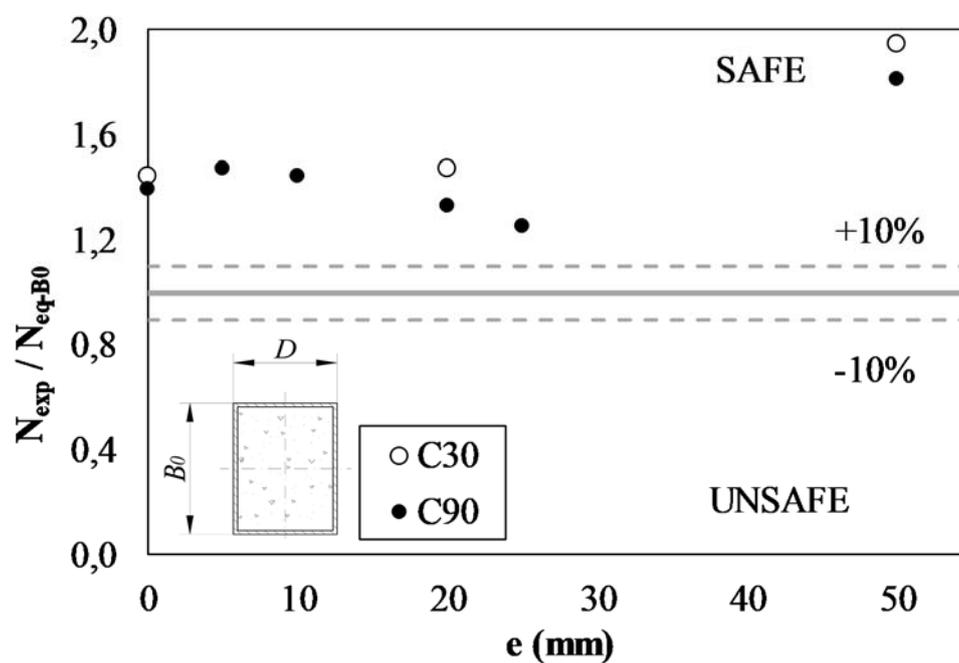
Fig. 15. Comparison between proposal B<sub>0</sub> predictions and experimental ultimate loads.
