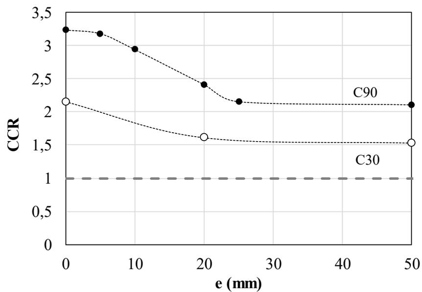
Fig. 8. Concrete contribution ratio (CCR) vs eccentricity.
