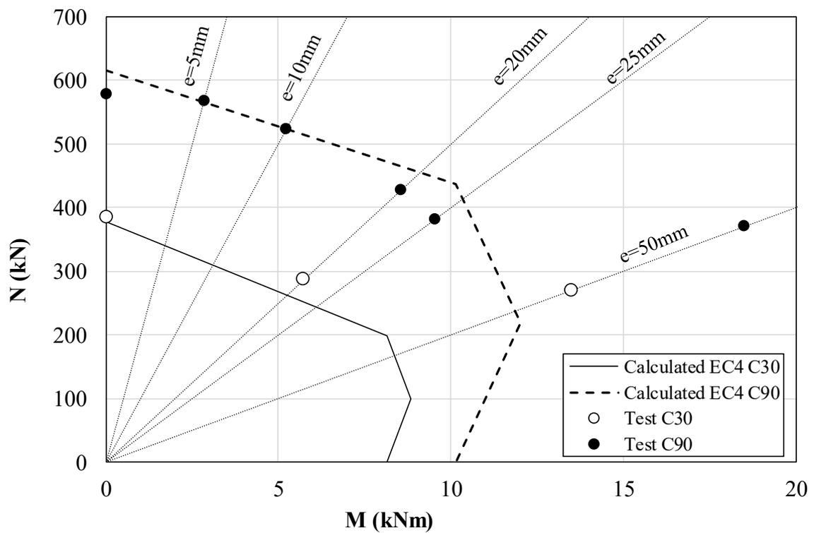
Fig. 11. Combined axial force-bending moment M-N interaction curve.
