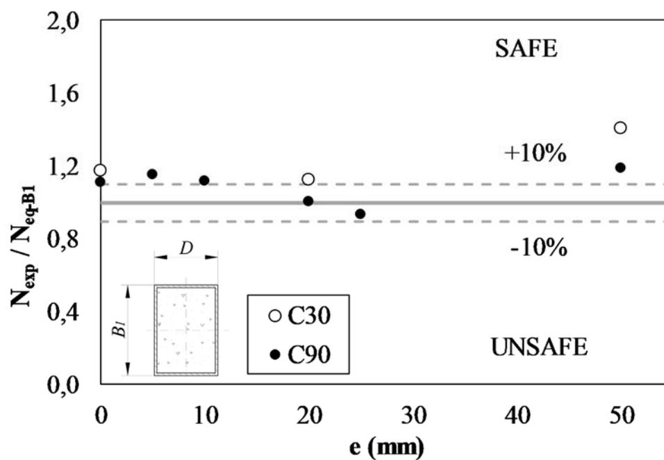
Fig. 16. Comparison between proposal B<sub>1</sub> predictions and experimental ultimate loads.
