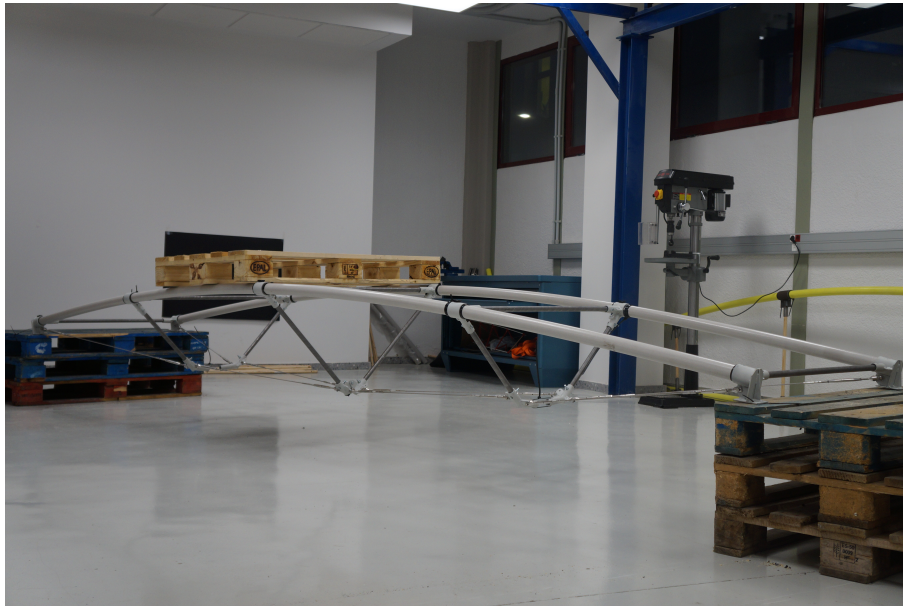
Figure 2: Experimental lightweight footbridge based on the active bending principle
