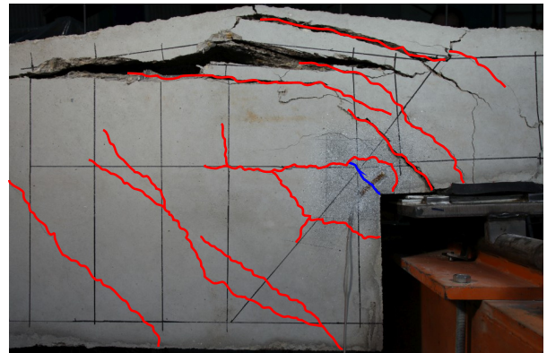
Fig. 7. Crack pattern for peak load represented in photos taken after peak load (in blue highlighted cracks at 30% V_u ).
