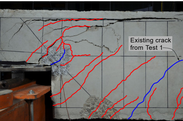
Fig. 7. Crack pattern for peak load represented in photos taken after peak load (in blue highlighted cracks at 30% V_u ).
