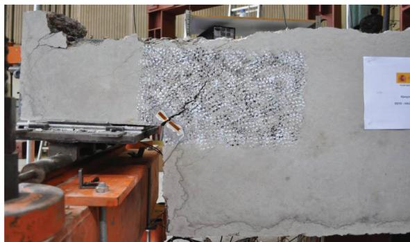
DETALLE DE RECUBRIMIENTO DESPRENDIDO
