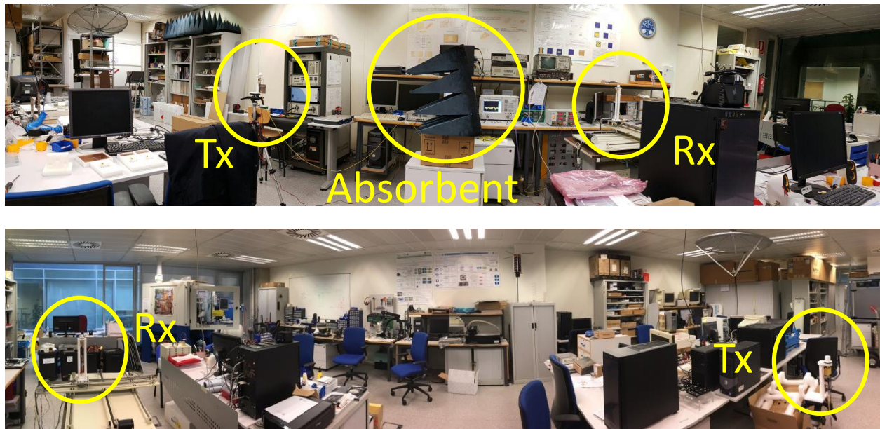
Fig. 2: Laboratory setup for the measurements. (Up) front view, where the transmitting antenna is on the left and the receiving antenna on the right, in the middle of the photograph the absorbent material used in a specific measurement configuration is shown. (Down) back view, where the transmitting antenna is on the right and the receiving antenna on the left.
